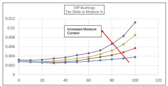
As can be seen, the higher the Moisture Content, the Tan Delta can reach very high Tan Delta values at Temperatures 60 to 90 Deg. Cent. and can result into thermal runaway and cause OIP Insulation & ultimately Bushing Failure.
