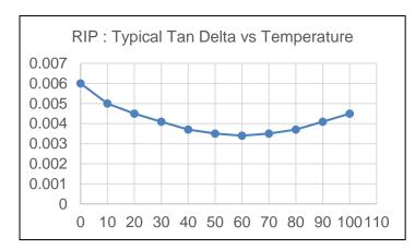
As can be seen from the graph, the RIP Bushing has lowest Tan Delta value at Temperature of @ 60 Deg. Cent. The Tan Delta keeps increasing as Temperature goes below 60 Deg. Cent. A similar Tan Delta behaviour is reported in RIS Bushings also with slightly lower values than in RIP Bushings. Based on statistical analysis of data on variations in manufacturing processes of OIP & RIP
