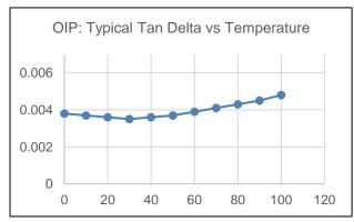
Typical Tan Delta vs Temperature Characteristics of OIP Bushings is shown in the Graph. As can be seen there is a variation in Tan Delta when the temperature is increasing. Lowest value is observed in between 20 Deg. Cent. and 50 Deg. Cent.
